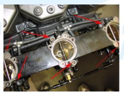
3.3 (Below) Turn the fuel switch to the off position. Remove three fuel inlet lines and one fuel return line. Remove the carbs from the hull.
