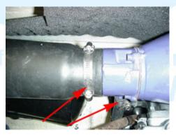
2.3 (Below) Remove the four allen head bolts securing the stinger pipe to the header pipe. Remove the stinger from the hull.
