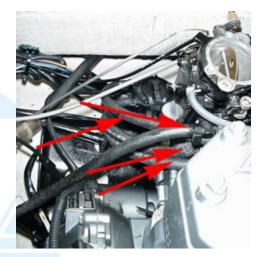
3.4 (Below) Remove the remaining pulse line and fuel inlet line from the fuel pump. Disconnect the two electrical quick connects. Disconnect the oil line.
