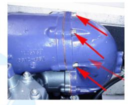
2.4 (Below) Remove the three allen head bolts and one nut securing the header pipe to the exhaust manifold. Remove the bolt securing the temperature sensor to header pipe. While removing from the hull disconnect the water line to the header pipe.
