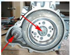
5.9 Remove the four bolts securing the seal plates to the engine and remove the plates. There are two of these plates, one on the front of the engine and one on the back of the engine. Remove the flywheel housing from the engine Your engine is now ready to ship to SBT.
