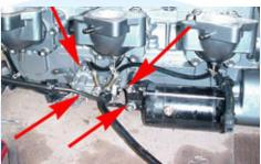
5.6 (Below) Place a rope in the cylinder to block the engine from turning. Using a wrench, turn the PTO counter-clockwise. (It is a regular thread and is very difficult to break free.)
