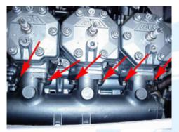
2.6 (Below) Remove the six studs from the engine that hold the exhaust manifold in place.
