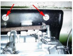
4.6 (Below) Flip the engine and bedplate onto its side and remove the four bolts securing the engine to the bed plate. Flip the engine and bed plate back and remove the engine from the hull.
