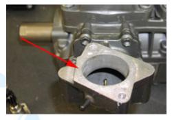
5.1 (Above) Remove the six nuts and twelve bolts securing the intake manifold to the engine. Remove the oil lines from the manifold.
