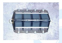
5.4 (Below) Look at each petal-to-cage surface and check for gap. If a gap of more than 0.015" is present, replace the petals.
