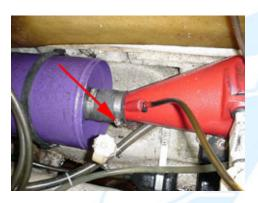
4.3 (Below) Remove the 11mm nut on the pipe clamp and remove the clamp from the pipe. Disconnect the two water lines from the pipe. This will allow you to remove the lower pipe section from the hull. Slide it back, tilting the forward section down to clear the exhaust manifold.
