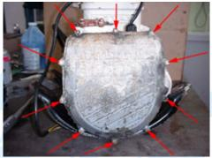
6.3 (Above) Remove the 10mm and 8mm bolts securing the flywheel cover and remove it.
