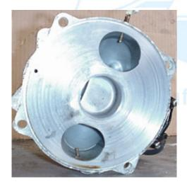
Examine the rotary valve itself. It must also be free of any imperfections. It must not have any pitting, holes, scratches, dings, dents, bends, etc. If any of these are present you MUST replace the valve.
