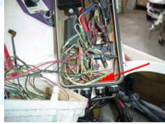
5.2 (Above) With the electrical box open, disconnect all the wires coming in from the flywheel assembly, and pull the wires out of the box. **NOTE: DO NOT CUT THE WIRES!**
