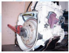
6.4 ( Above) Stuff a rag into one of the exhaust ports. Make sure the rag penetrates through the port, into the combustion chamber on top of the piston. This will prevent the engine from turning over while you remove the flywheel nut & PTO coupler. Remove the flywheel nut with a 14" pi pe wrench. A cheater bar may be necessary.
