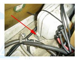
4.2 (Below) Remove the two 12mm bolts securing the lower pipe section to the exhaust manifold.
