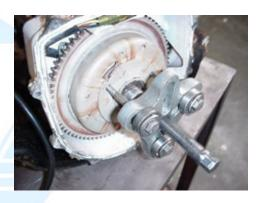
6.6 (Below) R emove the seven allen bolts fastening the flywheel cover to the block, and the three 4mm inner allen bolts securing the stator assembly. Remove them both.
