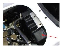
1.4 (Below) Disconnect and remove the oil catch can using a 10mm socket.
