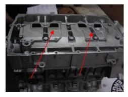
Notice the bottom of the engine has the oil pumps removed These DO NOT get sent to SBT with the engine. The oil pan does NOT get sent to SBT as well.
