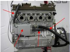
Remove starter, knock sensor and oil cooler.
