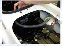
1.5 (Below) Disconnect the rear wire harness connections.
