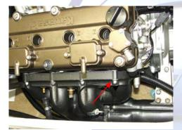
1.13 slide motor forward till it clears coupling and lift out of hull, until you can reach the lines on the bottom of the motor. Disconnect these lines
