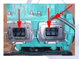
2.9 (Below) Remove the 12 6mm intake studs from the engine with a stud socket.
