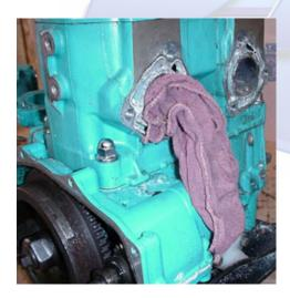
5.7 (Below) Use a chain wrench to remove the PTO flywheel.
