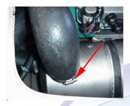
3.4 (Below) Remove the lower exhaust cooling line. Remove the exhaust pipe from the hull.
