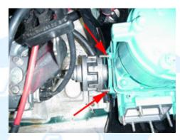
5.4 (Below) Remove the four 12mm nuts from the motor mounts, and slide the engine forward off the PTO coupler.
