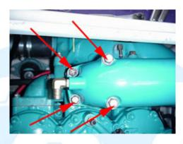
4.3 (Below) Remove the nine 12mm nuts securing the exhaust manifold to the engine and pull the manifold back off the studs.
