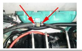
4.5 (Below) Remove the nine exhaust studs with an 8mm stud socket. Remove the starter ground and positive wires with a 10mm socket.
