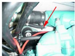
4.2 (Below) Remove the 12mm pipe to manifold bolts. Loosen the pipe to waterbox coupler and slide the pipe up and forward to remove it form the hull.
