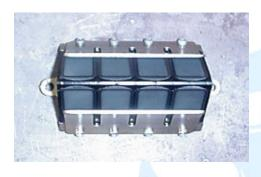
2.7 (Below) Look at each petal-to-cage surface and check for gap. If a gap of more than 0.015" is present, replace the petals.
