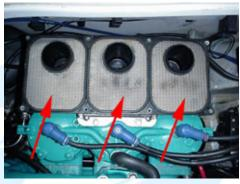
2.3 (Below) Remove the six 5mm allen head bolts securing the flame arrestor base and throttle bodies to the manifold and remove the base. Remove the throttle cable to the throttle bodies and quick connects to the throttle bodies. Remove the throttle bodies.
