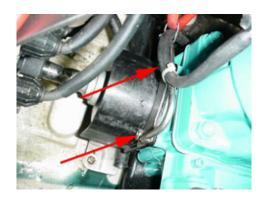
5.3 (Below) Remove the two PTO cover studs with a 6mm stud socket.
