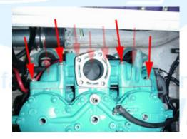
4.4 (Below) Disconnect the water lines from the manifold. Remove it from the hull.
