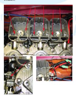
2.4 (Below) Remove the eighteen bolts securing the intake manifole to the engine. Remove the three oil lines to the manifold. Remove the intake manifold.
