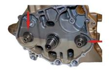
12) Once the oil tank is removed, the flywheel and starter drive gears can be removed. On the turbo version there are two counter balancer gears that need to be removed and kept for reinstallation.
