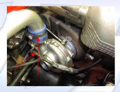
4) Blue coupler is removed from inlet tube and turbo along with the small wastegate hoses.
