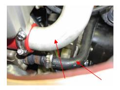
3) On turbo model, remove turbo intercooler tube and <sup>3</sup>/<sub>4</sub> black rubber hose beneath it.
